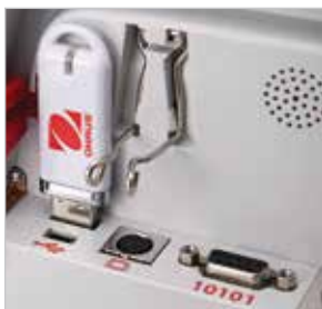
USB host and device ports, RS232, optional Ethernet, optional 2 nd RS232
