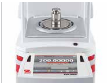
Calibration is easy with internal AutoCal™ or manually with an external mass
